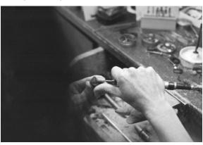
**Step 5:** Attaching a wire wax to serve as a sprue is the final step before casting or creating a pattern.
