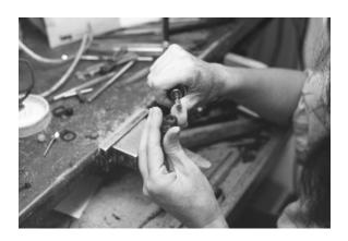
**Step 10:** A wire wax is attached to the finished wax design to ready the piece for casting or to make a model.
