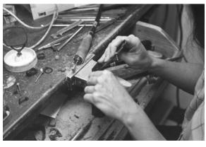
Step 2: A rough cut is made using a jewelers saw.
