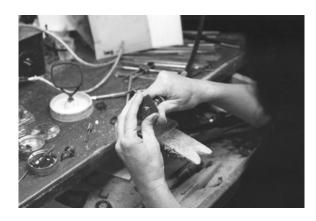
**Step 8:** Shaping a properly sized bezel can be also accomplished using a wide range of power or hand tools.
