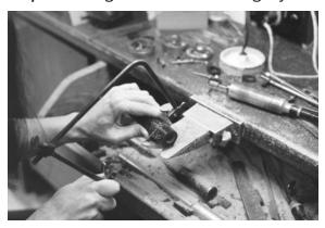
**Step 3:** Filing down the Ring Tube segment creates the rough shape of the finished piece and readies the piece for design work.
