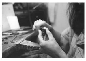
**Step 9:** The stone is test fit in the bezel to check rough seating, positioning and overall design aesthetics.
