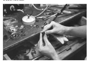
**Step 6:** The hole is cut into the File-A-Wax piece using a motor tool. This can also be done with a carving knife.
