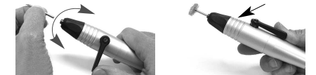
Turn lever 90° to left or right to open collet and release bur
